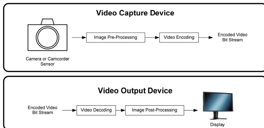
**Figure 1: Basic block diagrams for video-capture and video-output devices showing where video pre-processing and post-processing occur.**
