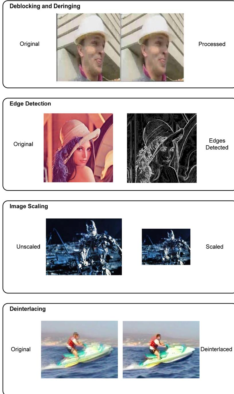
**Figure 3: Examples of four post-processing algorithms: deblocking and deringing, edge detection, image scaling, and deinterlacing**
