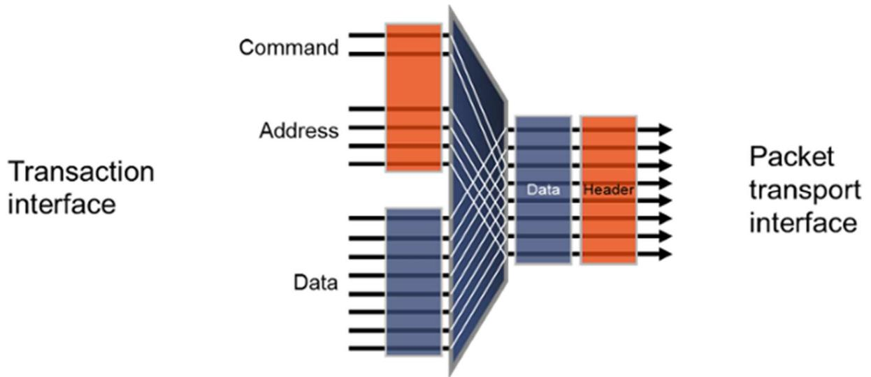
**Figure 1: Packetization places the address and control signals on the same wires as the data.**
