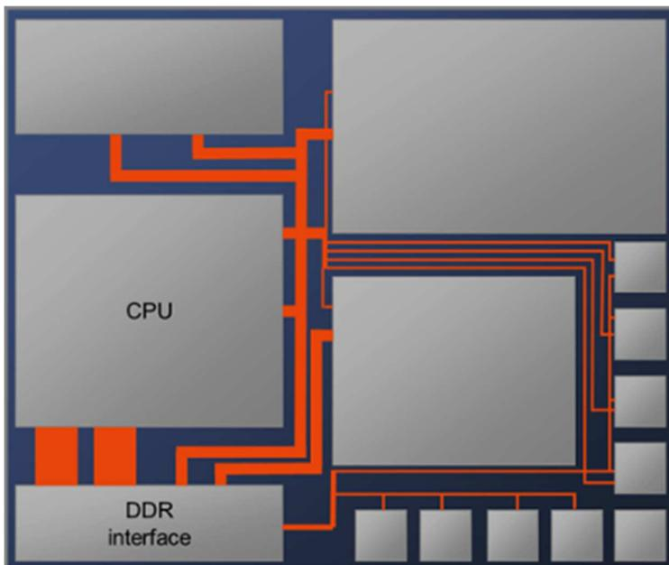
**Figure 2: Packetization and serialization reduce the total wire length of the top level interconnect by 50%.**
